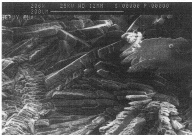
Fig. 1 Heavy zinc phosphate conversion coating crystal morphology
